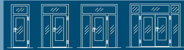
Floor to ceiling glazed doors with over-lights shown as single or double door arrangements
